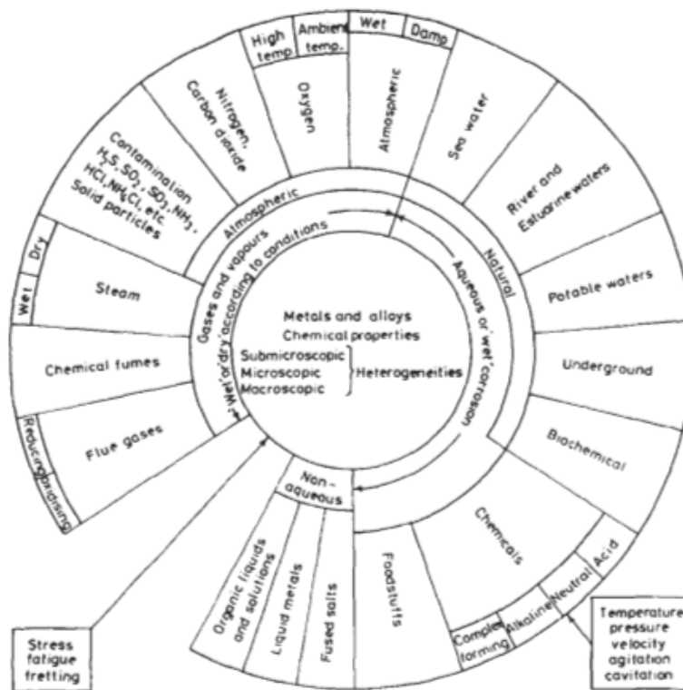
Fig.1.3 Environments in corrosion
